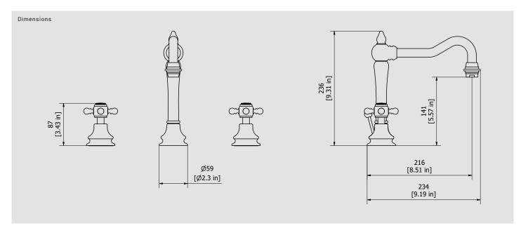
Cartridge Threaded fitting IB G1/2" ceramics headworks Treaded fitting G1/2" male Aerator Flow Rate (+/-10%) 1 BAR 2 BAR 3 BAR M24x1 perlator coin slot 9.5 l\m 14 I\m 17 I\m
