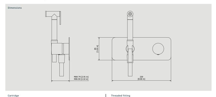
G1/2" female Ø35 ceramic cartridge Aerator Flow Rate (+/-10%) 1 BAR 2 BAR 3 BAR 2.3 I\min 3.2 I\min 4 I\min
